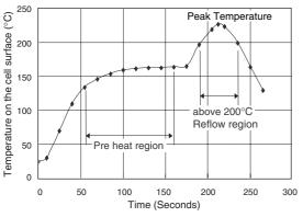
The times of repeated reflow soldering must be two times or less. The Temperature must be measured at top of the cell.
