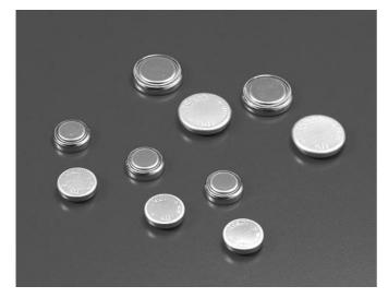
TS(Titanium Silicon) Lithium-Ion battery is 1.5V type rechargeable battery features large capacity, wide charging voltage range, long cycle-life and excellent reliability with using titanium composite oxide as cathode and originally developed Litium silicon oxide as anode.
