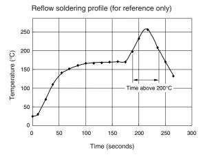
The times of repeated reflow soldering must be two times or less. The Temperature must be measured at top of the cell.
