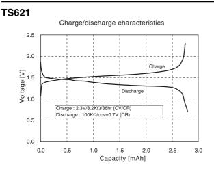
Charge voltage dependence of discharge capacity
