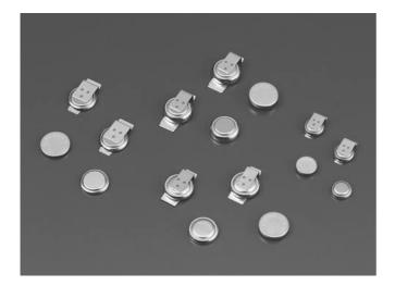
Using chemically-stable large surface area activated carbon as electrode, this new type of capacitor features highcapacitance, low-impedance, high-rated voltage, and long-term reliability through unique sealing technology. Moreover, using original heat resistant materials and cell design, the capacitor allows reflow soldering in response to the demand of automatic mounting.
