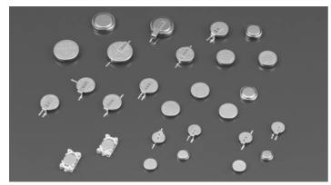
SII own developed MS(Manganese Silicon) Lithium-ion rechargeable battery addresses the demand most effectively. The battery uses silicon oxide as anode and lithium manganese composite oxide as cathode. As a result, it offers twenty times the capacity of conventionally available batteries, in addition to longer cycle-life and highly stable over-discharge characteristics.
