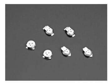
RB Lithium-Ion rechargeable battery allows reflow soldering for automatic mounting, by adopting highly heatresistant material and precise sealing technology. RB Series features high capacity and long cycle life with possible charging voltage range from 1.8V to 3.3V, which is most suitable for backup use of real time clock and SRAM etc.
