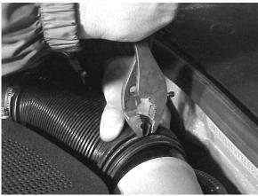
Step 7: Detach upper half of airbox from lower half by unhooking metal clips. Clips pop outwards with flat head screwdriver. There are 4 clips around perimeter of box. Rehooking the rear clip on engine side of airbox during re-installation is easier done with long screwdriver or prybar.
