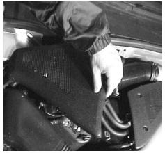
Step 2: Remove air box ducting by pulling upwards and outwards.
