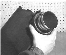
Step 12: Reinstall MAF and factory o-ring. Seat sensor by wiggling into air box opening. Closing metal clips will pull MAF flush to air box. A little soapy water around the flange of the MAF can help here. Do not use petroleum based lubricants!
