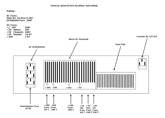
The AC Distribution block on the left (comprising of  $3 \times IEC$  connectors) is not fitted to the 16-channel add-on modules.
