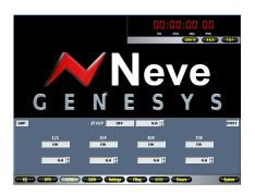
Allows setup and control of the 2T paths from the 8T Groups.
