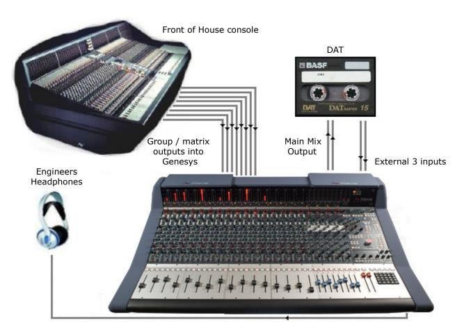
While the output for the main Front Of House console may be of a high standard, the mix created for the venue does not have the correct balance for a live recording. Genesys solves this problem.
