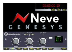
If an EQ is being used to be the Sidechain into the Gate (or Exp), it will no longer be available in the Channel (or Monitor) path.
