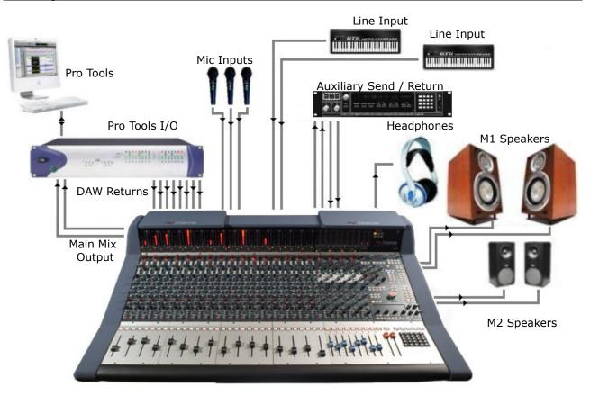
Genesys can be used to monitor from the workstation while recording directly from Mic or Line inputs.
