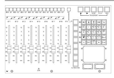
The 8T faders can either control the 8T levels or a block of 8 DAW faders (the red led underneath the faders will light when DAW control has been established).
