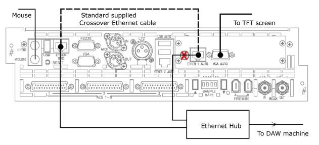
The dotted lines show the two Ethernet ports connected when the unit is not connected to Pro Tools or an external DAW (this will mean that the console cannot control HUI paths). This cable should always be fitted if not controlling a DAW.
