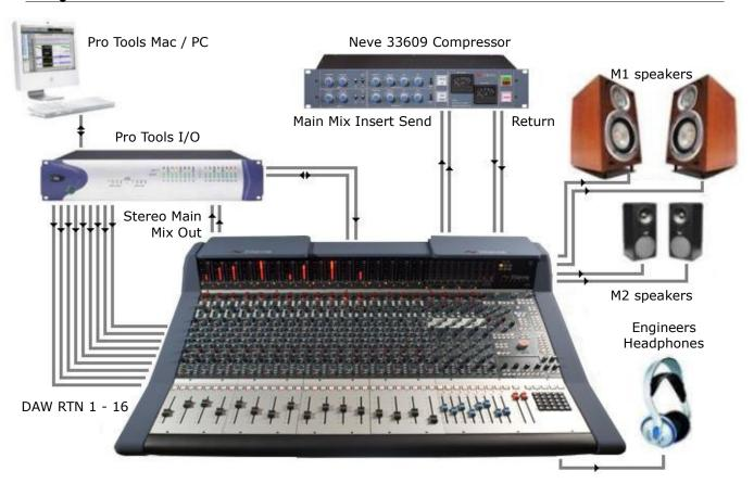
Connect the outputs of the workstation to the inputs of Genesys.
