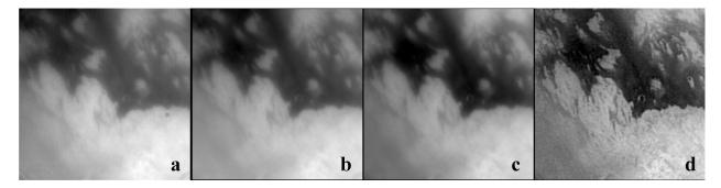
**Figure 2:** Processing of a regional scale Titan image: (a) shows the raw image; (b) shows the same image once radiometric calibration, flat-fielding, and despiking have been performed; (c) shows the same footprint with three frames summed together; and (d) shows the final result once a sharpening procedure had been applied. Image used: N1481618305, 812 m/pixel, CB3 filter, target distance=70662 km, phase angle=16.4 degrees. For summation, images N1481618211 and N1481618243 were used.
