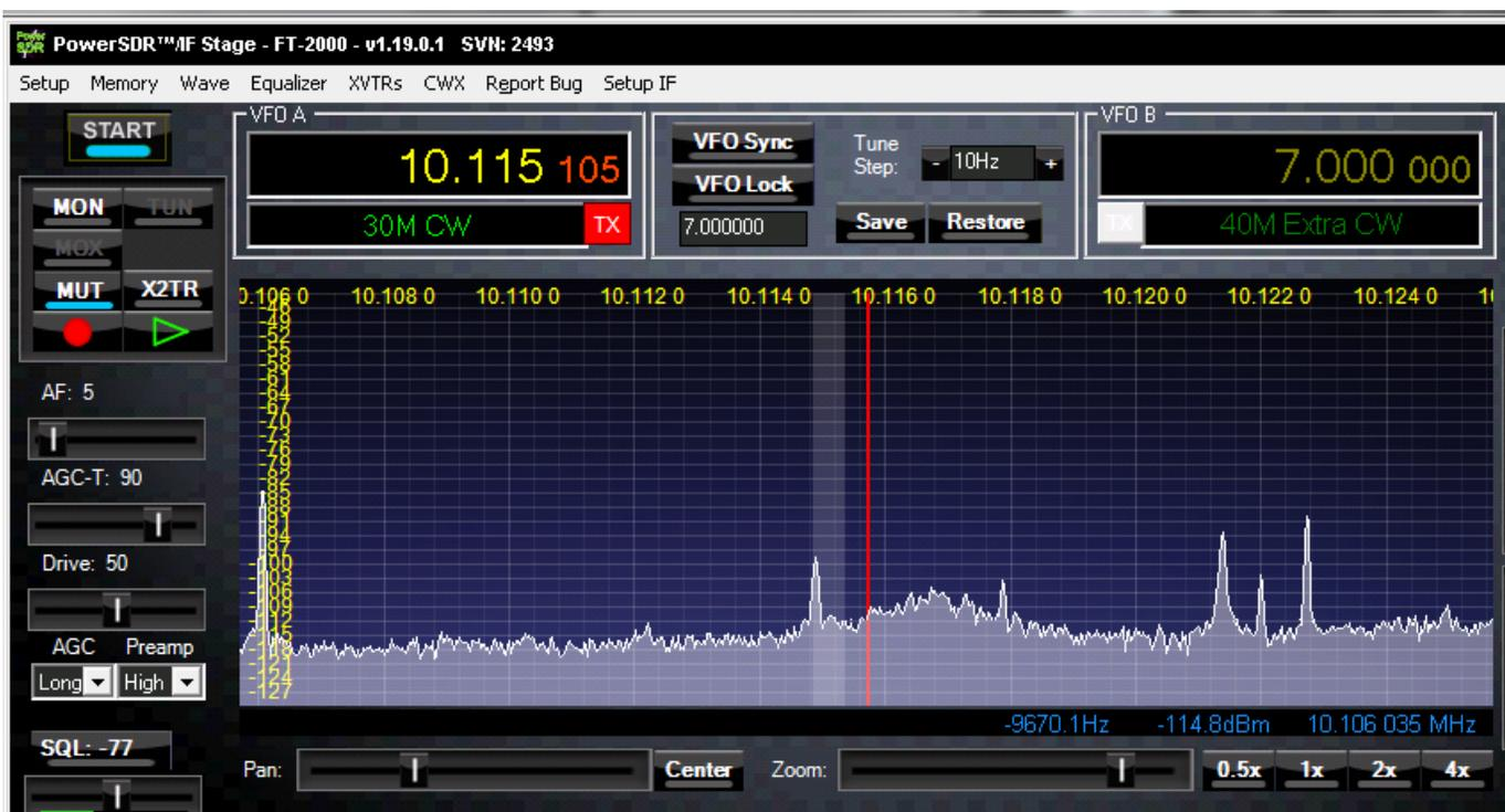
You should see some movement on the panadapter part of the screen. As you tune the radio to signals using the knob, we hope you will see some indication of these signals on the PowerSDR screen – even though they may not line up with the proper locations. That lets us know things are working at a basic level.
